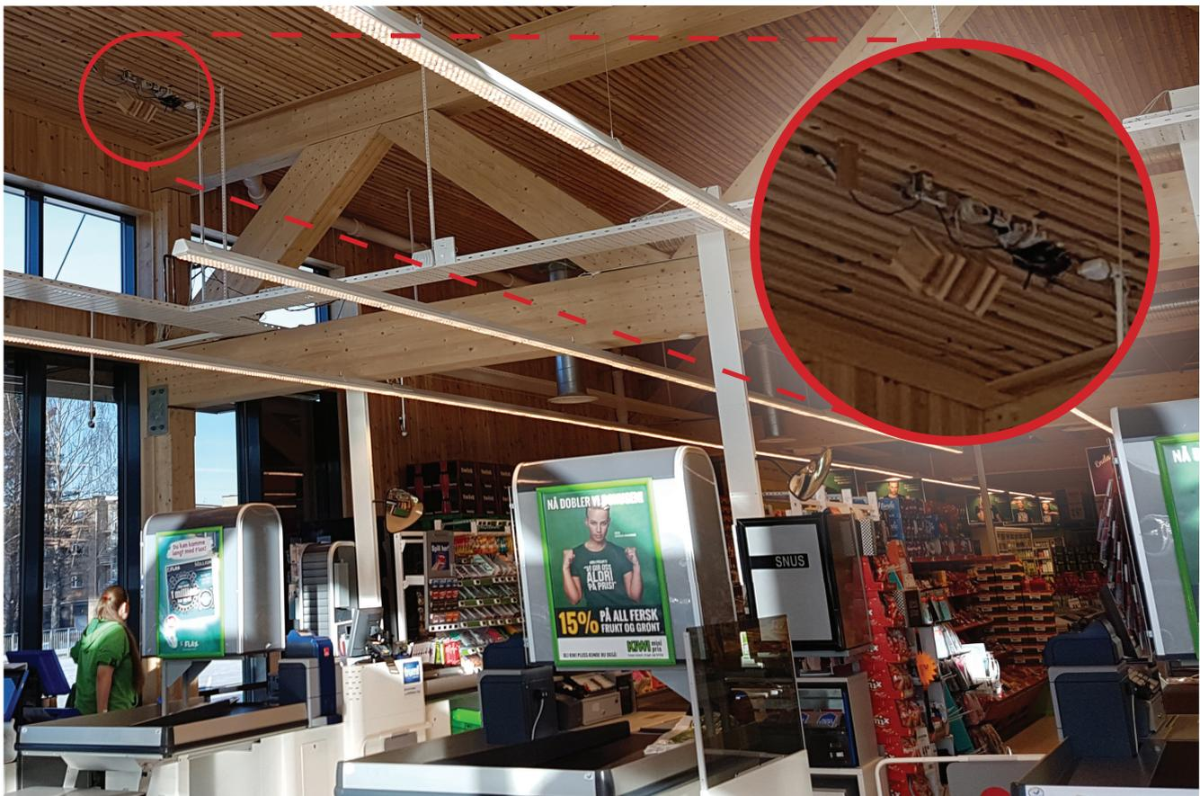
Figure 1. Monitoring of moisture buffering effect of wood material at the Supermarket Kiwi Fjeldset at Elverum in Norway. Image Kristine Nore, Norsk Treteknisk Institutt.
