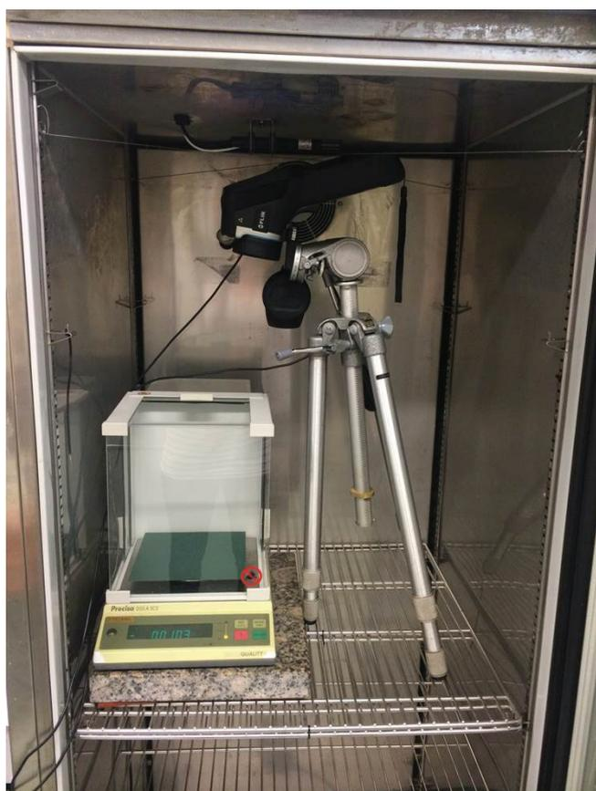
Figure 5. Experimental arrangement to measure surface temperature rise
