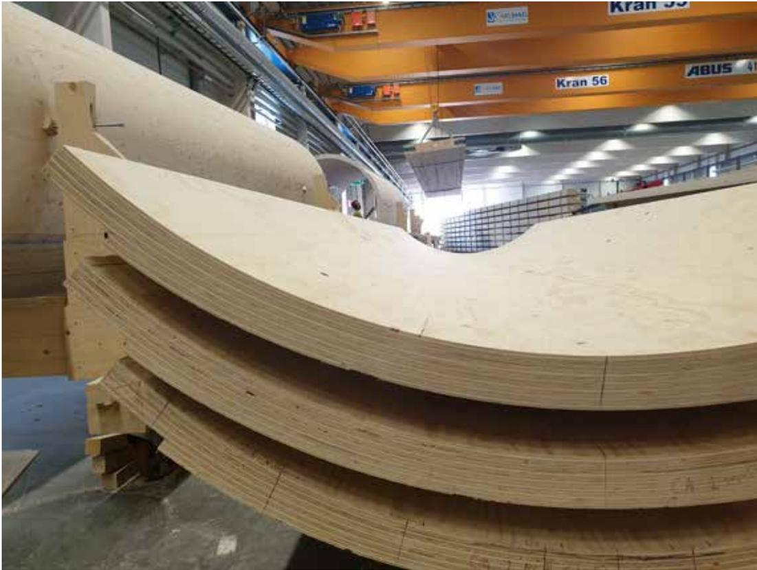
Stacking the wooden elements on top of each other means you can efficiently transport wind towers to places that used to be unreachable with steel structures.
